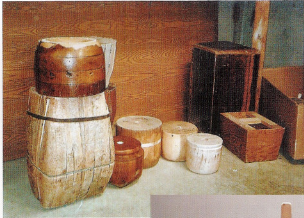
Left, various basket molds, these are over 100 years old. Below, basket molds used by today's basketmakers.
